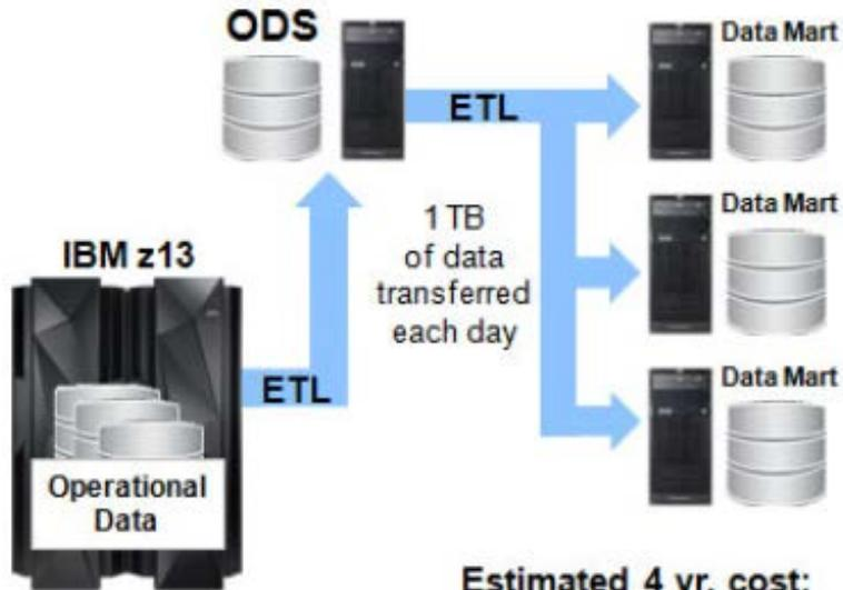
Assuming four cores on z13 running at 85% utilization and 12 cores on x86 servers run at 45% utilization, ETL activity burns **519 MSU** and uses **10 x86 cores** *per day*.
